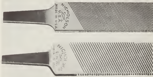
2-44. An illustration which shows the difference between a single-cut and double-cut hand file. (Nicholson File Co.)
